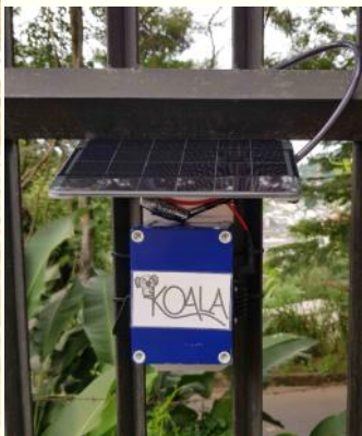
A QUT-KOALA Air Quality Monitor installed in Kandy
